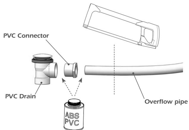
**NOTE:** If necessary, cut the overflow pipe to the desired length, and glue it to the PVC connector and to the drain.
