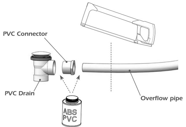
**NOTE:** If necessary, cut the overflow pipe to the desired length, and glue it to the PVC connector and to the drain.
