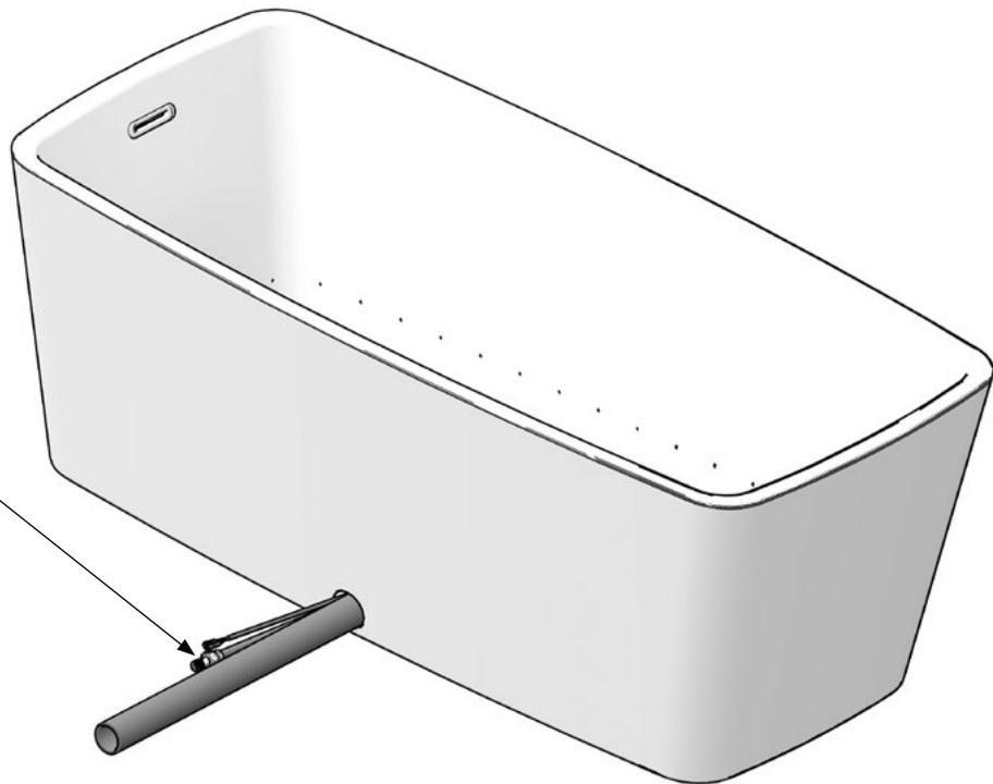
(\*): The location of the air conduit is shown as an example. It may differ depending on the positioning of the remote components and the orientation of the bath.
